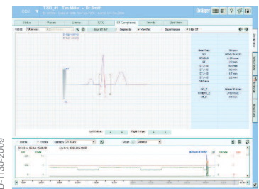
ST Complex screen Displays zoom-in on median complex showing ST-related caliper measurements
